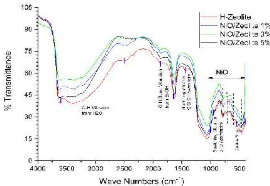
**Figure 2.** FTIR spectrum of H-Zeolite and NiO/Zeolite 1%, 3% and 5%
