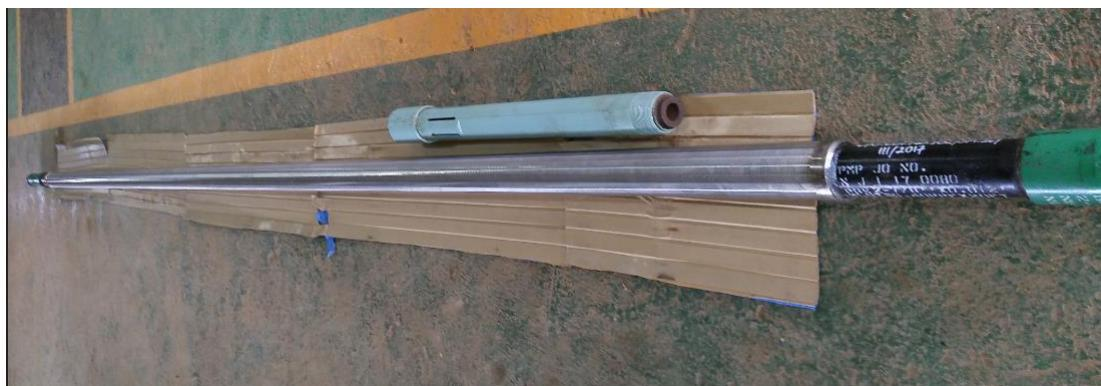
Figure-9. Comparison between sandtrap vs wire-wrapped screen with PBS 2-7/8"
