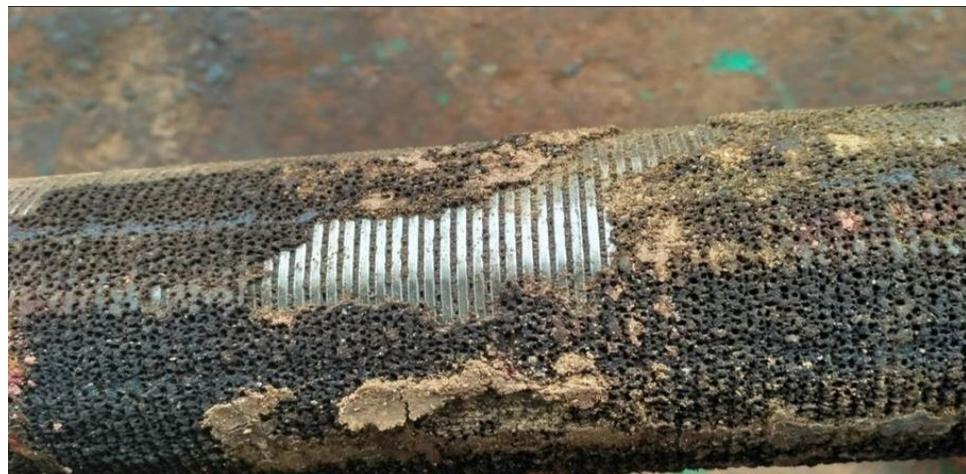
Figure-10. Wire-wrapped screen liner covered by sand and other solid materials on its outer surface after pulling out during well service at ASD-14
