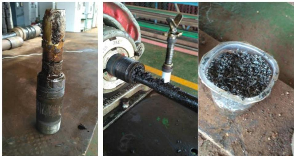
Figure-7. Sand inside the tubing pump during routine WS findings at ASD-14 well
