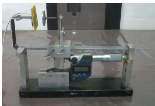
Gambar III.1 Alat kalibrator jarak
