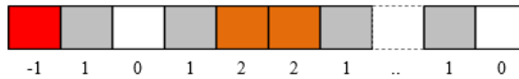
Figure 4. Number notation for row matrix at each layer of the roast process composition (-1: heater; 0: air in the vacuum chamber; 1: sand; 2: food/roast object).
