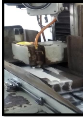
Gambar 3. Proses grinding surface
