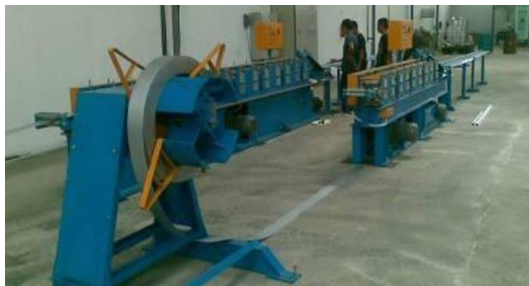
Gambar 7. Roll Forming Machine
