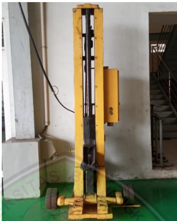
Gambar 1. 1. Dongkrak Lokomotif ( Lifting Jack ) Sumber: KAI (2022)
