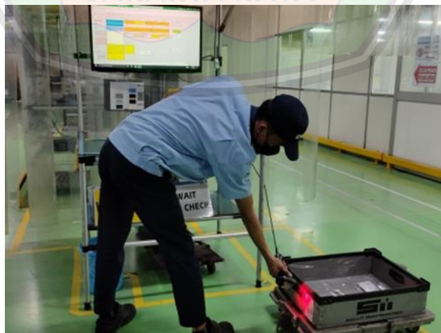
Gambar 1.3 Posisi Badan Saat Proses Scan Barcode Small Part Sumber : Dokumentasi PT Indonesia Epson Industry (2022)
