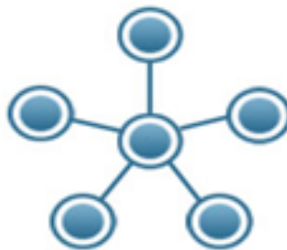
Gambar 2.3 Model topologi bintang
