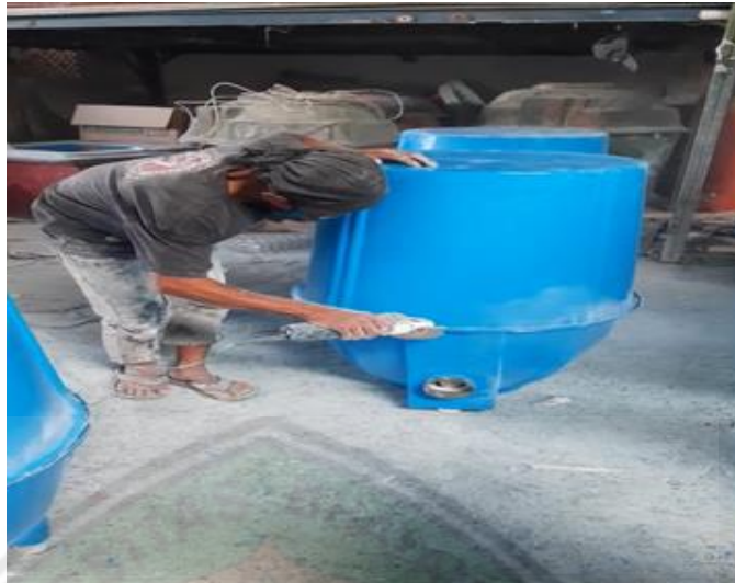
Gambar 1. 1 Proses Finishing Septictank Fiber
