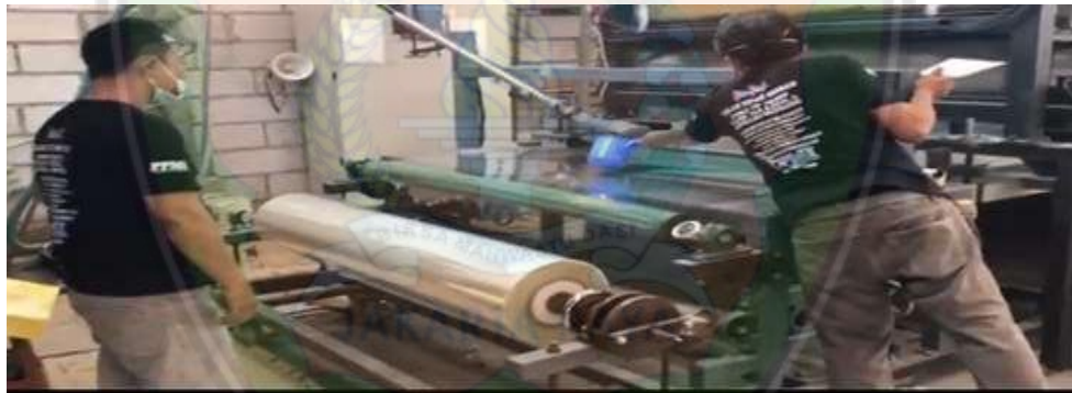
Gambar 1. 1 Proses Pemberian Polimer Resin
