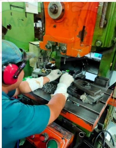
**Gambar 4. 1 Proses *Notching***
