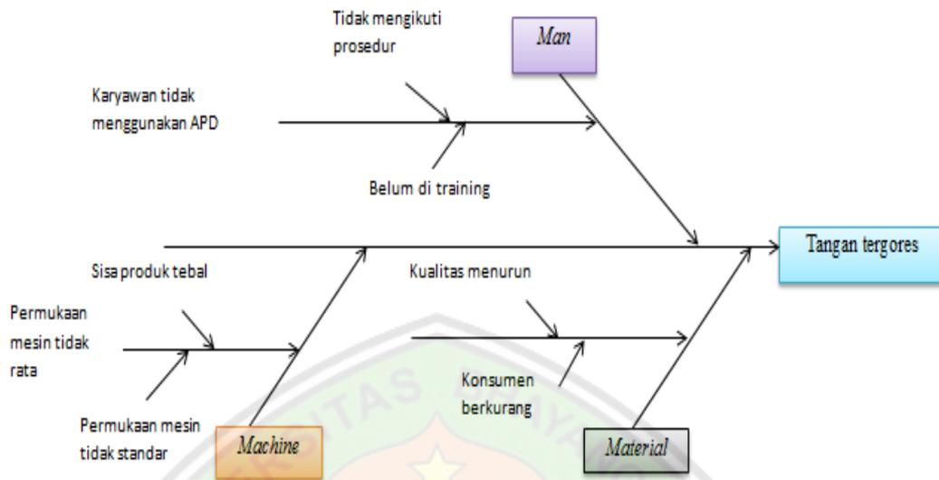
**Gambar 4. 6 Diagram Fishbone Tangan Terjepit**
