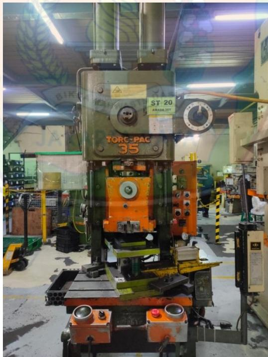
**Gambar 4. 3 Mesin *Notching***
