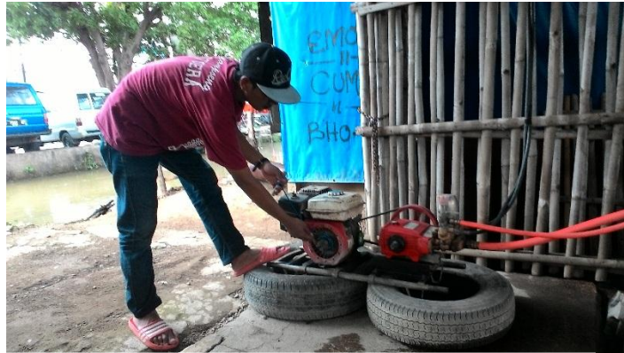
Gambar 1.1 : Proses Pengoperasian engine spray
