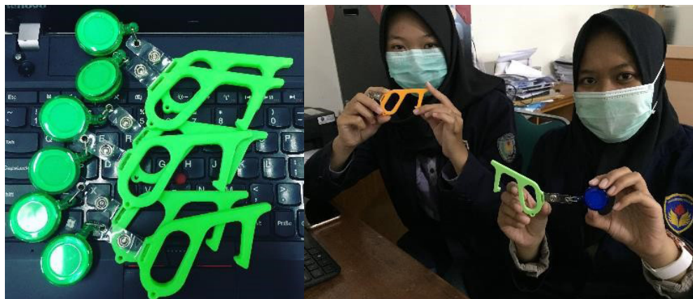
Gambar 5. Hasil 3D printing alat safety finger extension .
