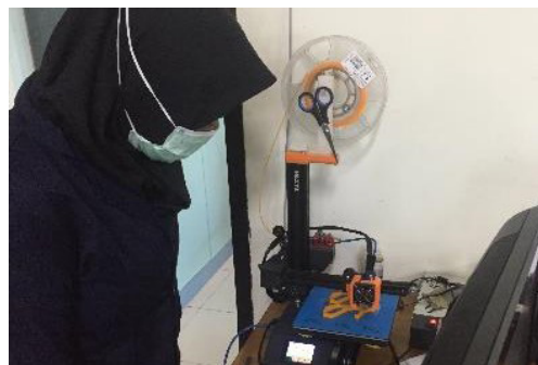
Gambar 4. Proses 3D Printing alat safety finger extension
