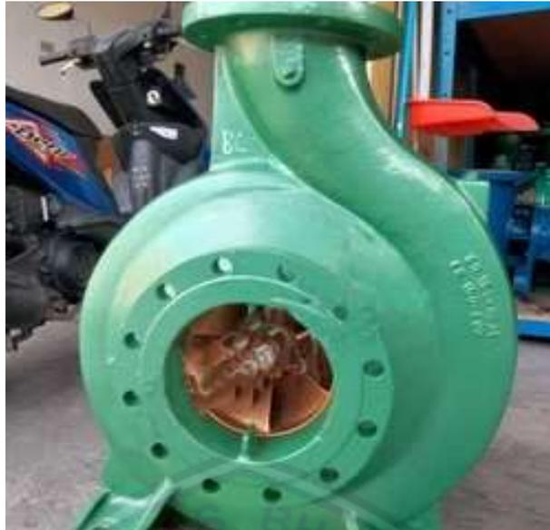
Gambar 1. 1. *Casing* Pompa Sentrifugal
