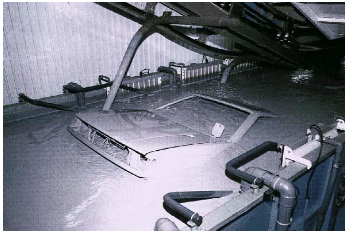
Gambar 1.1 Proses pengecatan dasar model celup ( dipping )
